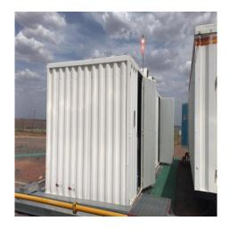
Utility integrated equipment includes instrument air and desalting water system. The split skid design makes the movement and transportation more convenient
