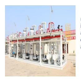
MDEA aqueous solution is used to remove CO<sub>2</sub> from the feed gas in the integrated equipment of pretreatment and purification, and the acid gas is desorbed by depressurization heating after adsorption
