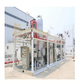
MRC liquefaction process is adopted in the integrated liquefaction equipment, which uses mixed refrigerant, exchanges heat with gas in the cold box, adopts two-stage refrigeration gas liquefaction technology with lower energy consumption
