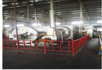
Horizontal chain furnace: Pipe primer curing, accelerate setting and adhesion of coating, 150 pcs/shift
