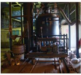
Sandblasting machine: Sand blasting on the inner wall of pipes, treatment of oxide and alkali layer on the inner wall, 80 pcs/shift
