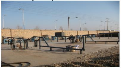
Internal and external wall rust removal: Self-designed internal and external wall rust removal machine, 350 pcs/shift
