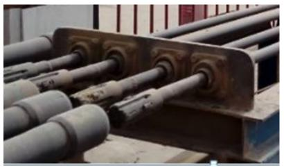
Alkali scale cleaning equipment: Unique design of knife head, effective response to thick alkali scale, 1 pcs/2 min
