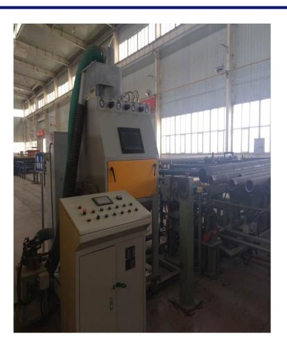
Shot blasting machine: LW/PS1-YG7 can realize surface treatment of tool threads below 10"to meet the technical requirements of surface treatment.
