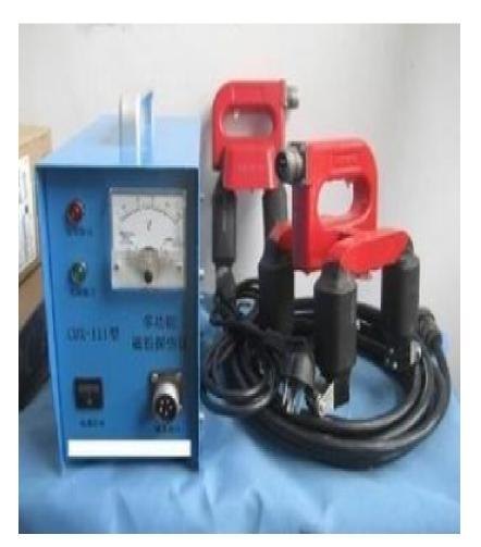
Nondestructive testing equipment: The magnetic particle flaw detection machine is specially designed for the detection of threads at both ends of tubing and casing short joints.
