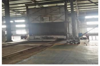
Finished product curing furnace: Pipe finish curing, adjust temperature, accelerate condensation of coating, 300 pcs/furnace
