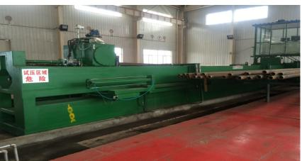
BCH/SY-114 hydrostatic pressure tester: 2 sets
