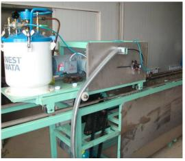
Spraying equipment: Inner wall spraying, uniform coverage of pipe wall, 100 pcs/shift
