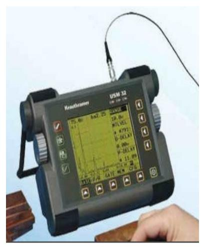
Nondestructive testing equipment: Ultrasound flaw detection machine is specially designed for the flaw detection of tubing and casing short joints.
