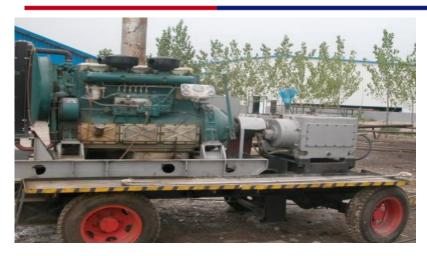
High-pressure cleaning machine: Adjustable and controllable pressure 10-40 MPa, cleaning effect of tubing and casing is remarkable with high efficiency.
