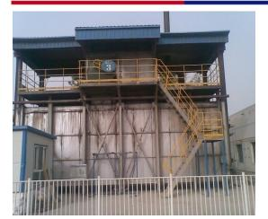
thermal cleaning Furnace: Radiation heating 200-400 °C, carbonized loosening on heavy oil and alkali layer, 300 pcs/furnace
