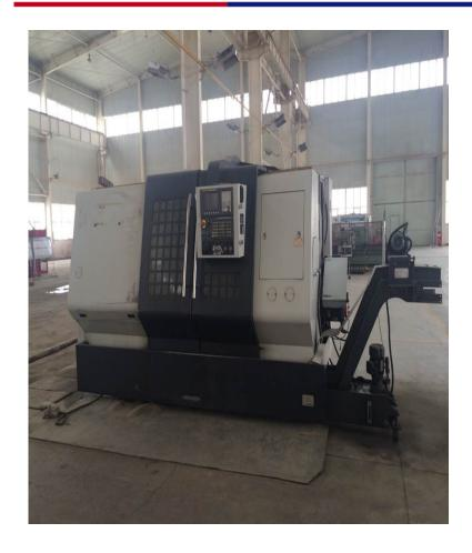
CNC lathe: HTC5020B (60.32-114.3mm) quantity: 2 sets, mainly for tubing short joint processing, coupling processing.
