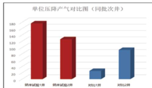
Comparison Chart of Gas Production per Unit Pressure Drop (Wells from the same batch)
