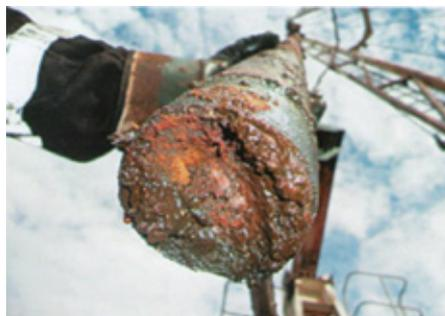
73mm diameter uncoated tubing removed from the well during workover
