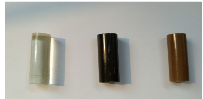
CCA100 (left) and special polymer plugging agent with different solid powders
