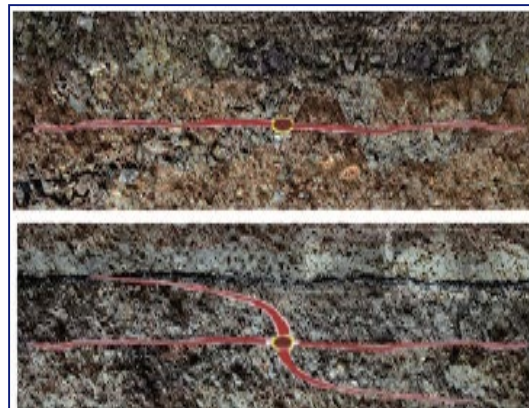
2. Diverting fracturing by temporary plugging of fracture opening
