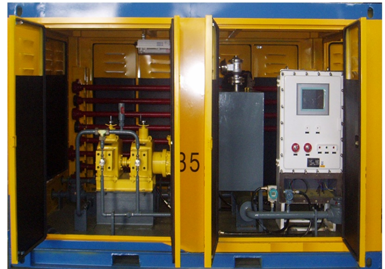
The foam generator
